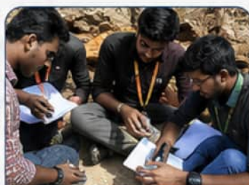
📐 Measuring strike and dip using Brunton compass
